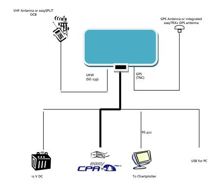
Schematics for the easyCPA-Alarm connection
