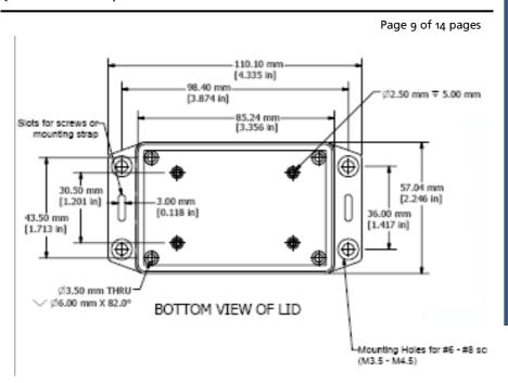
mounting template with hole positionte
